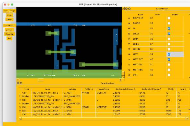
Figure 58: Use-case for gcd1_ERC008: bottom VPWR row removed (68/20).
