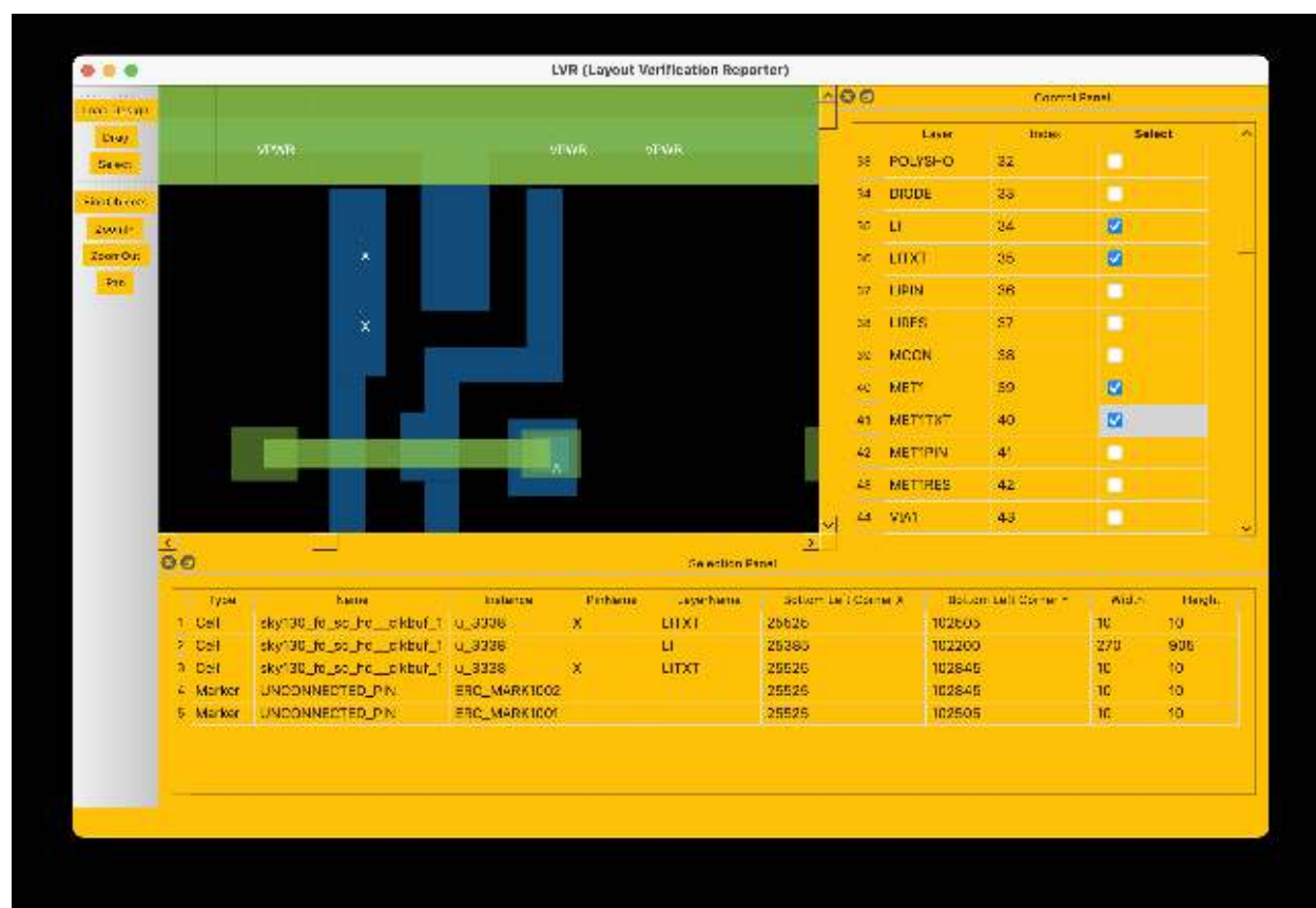
Figure 4. Connectivity view during ERC review. Shapes coloured by net; the Selection Panel reports the nets and pins involved.
